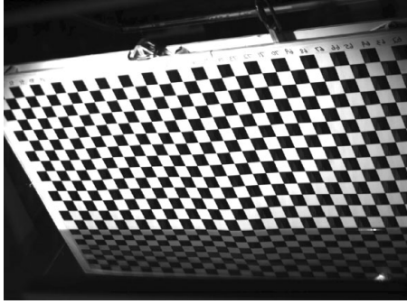
FIGURE 9. A photograph of the calibration chequerboard with its surface in the plane of the light sheet.
